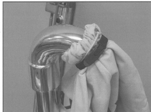
27. Secure dust bag on elbow.
