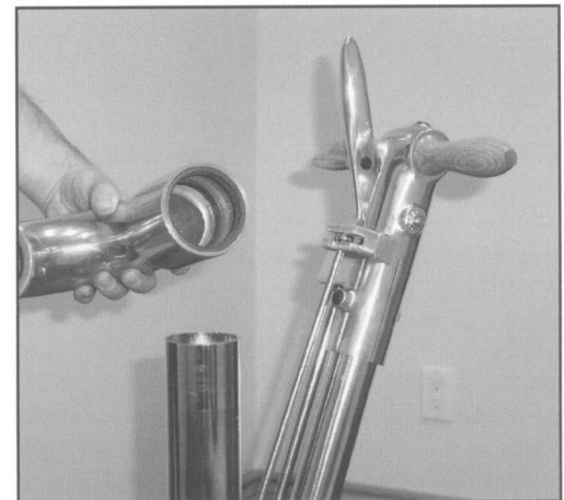
40. Clean out dust accumulation between the seals.
