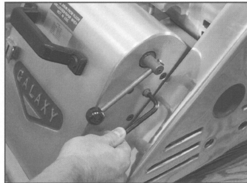
26. Turn adjustment screw as required.
