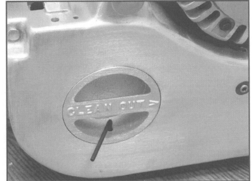
39. Use the key provided to remove dust cover.
