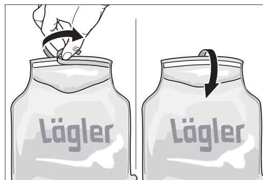
Fig. 15 Pull cover from the adhesive strip and seal the bag. The dust bag must be deposited in the open air!
