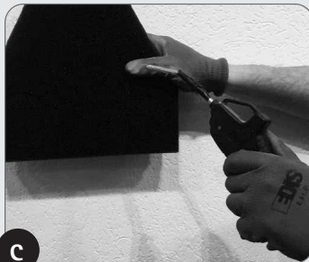
Blow the filter with an air gun
